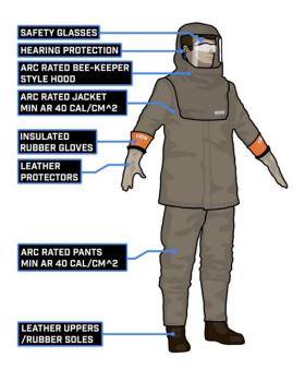
For accessing any equipment with a nominal voltage of greater than or equal to 1000V, the NFPA 70E Table 130.7(C)(15)(a) indicates that AF PPE Category 4 shall be worn.
